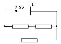
The total power dissipated in the circuit is 36 W. What is the emf of the cell and what is R?
